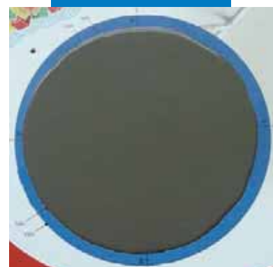
Checking the fluidity with a vibro-board
