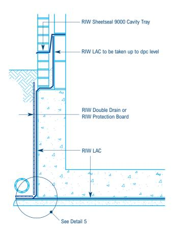
Minimum 20mm mortar fill in **DETAIL 3** conjunction with inner leaf **INTERNAL TANKING RIW LAC** RIW LAC lapped / sealed with dpc Masonry supporting wall **RIW LAC** Screed or Floating floor finish **RIW LAC** Λ Loading screed / slab as required າກົດການ See Detail 6 RIW Sheetseal 9000 dpc
