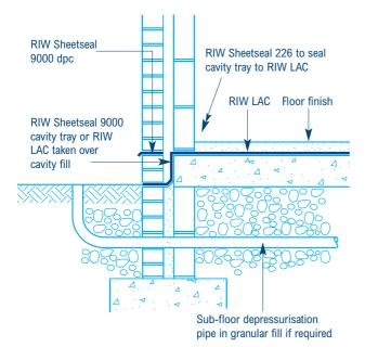
DETAIL 5 EXTERNAL TANKING ANGLE DETAIL (see detail 2) RIW LAC
