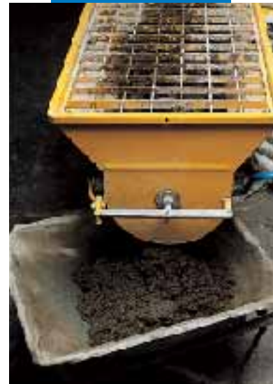
Mixing Mapecem in a mini-batcher
