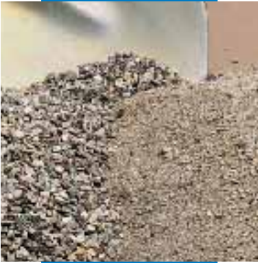
Aggregates for Mapecem: gravel from 4 to 8 mm and sand from 0 to 4 mm
